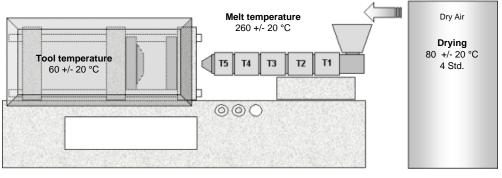
Typical filling pressure: Typical holding pressure: Typical holding time: 500 bar absolute +/- 25% 60 % of filling pressure 2 sec/mm wall thickness
