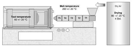
Typical filling pressure: Typical holding pressure: Typical holding time: 500 bar absolute +/- 25% 60 % of filling pressure 3 sec/mm wall thickness
