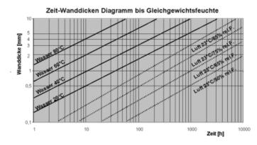
Polyamides are changing their glass transition temperature as a function of the humidity absorbed and hence some mechanical properties. The moisture absorption is depending on the storage conditions, time and wall thickness. The diagram shall give some base values about moisture pick-up. For any accelerated conditionning, the specialists of PENTAC Polymer may give you some further advise.
